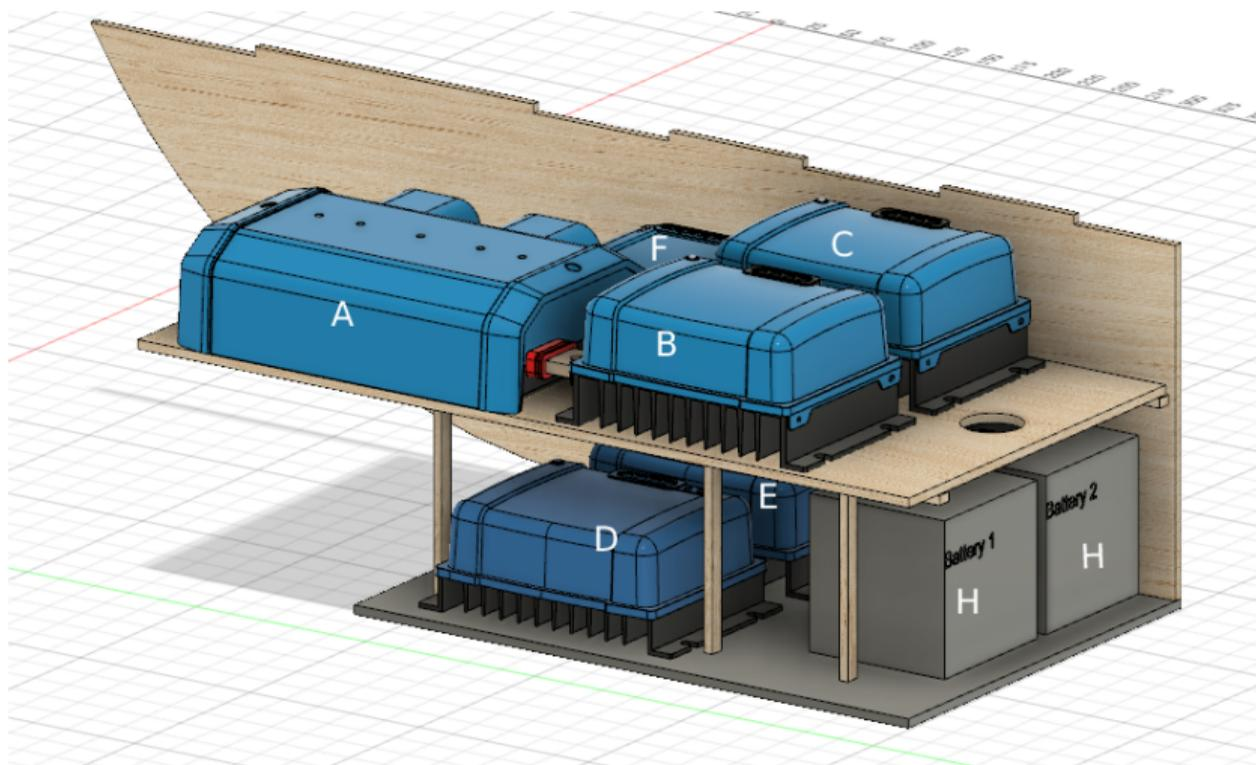
Solar inverters, chargers and batteries.
