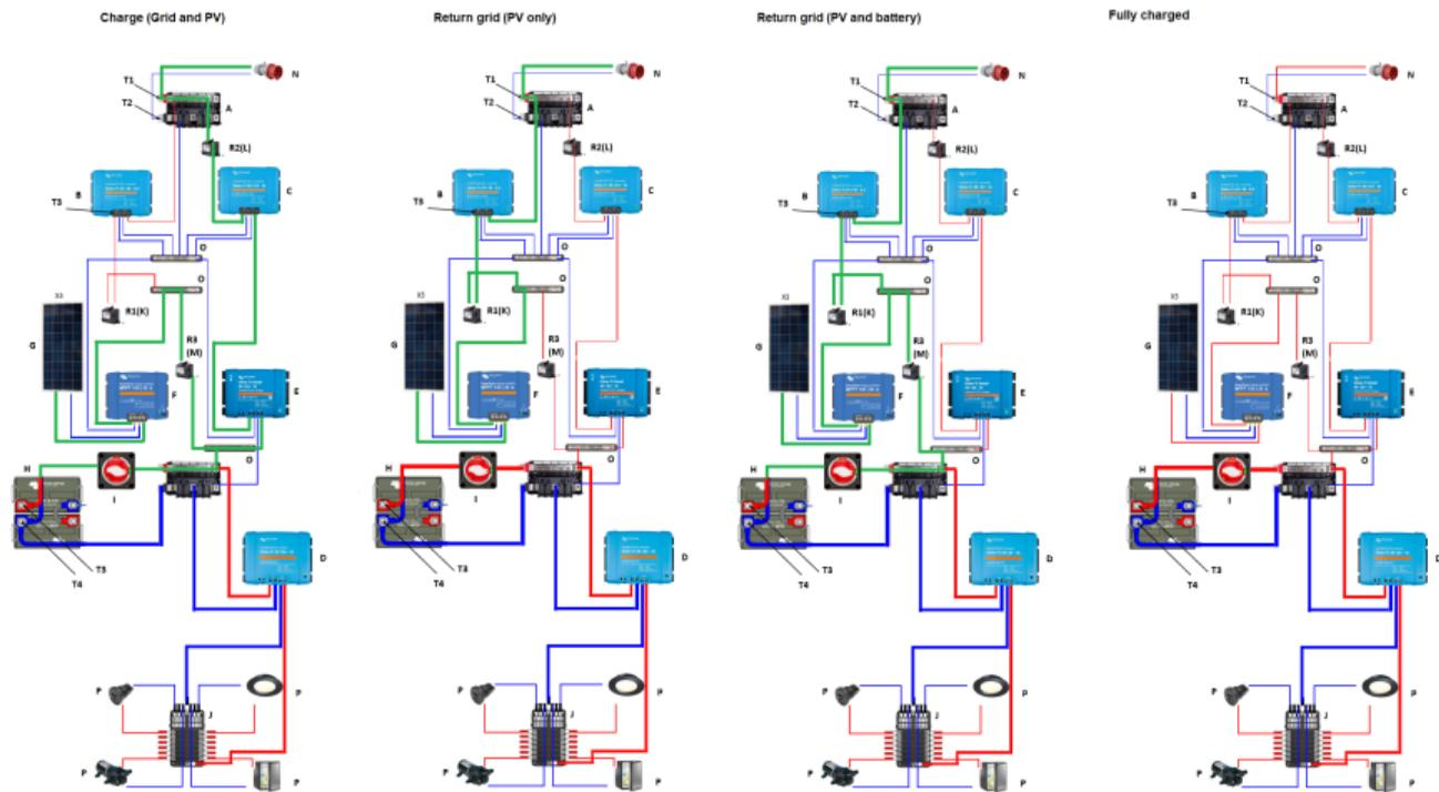
The four connection diagrams with contactors to control the DC grid operation.
