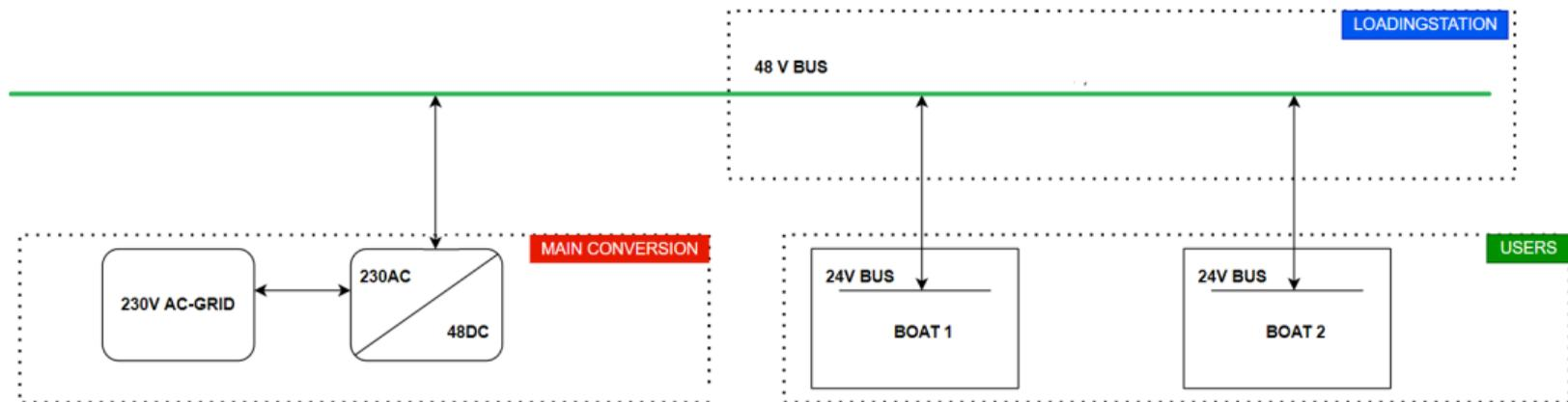
System overview, the green line includes the 350 volt DC grid with bidirectional conversion to the 48 volt DC grid.
