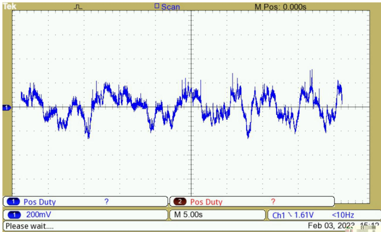
AC coupled measurement of the dc grid voltage
