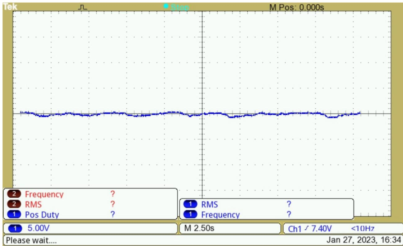
DC coupled measurement of the dc grid voltage
