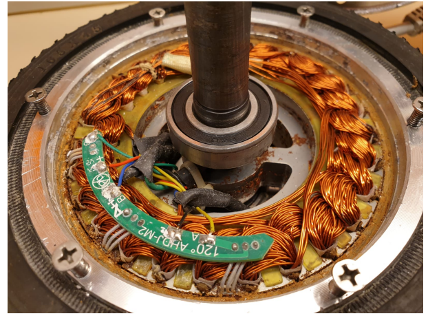
Fig. 3. View on the inside of a brushless motor to show the position of the Hall sensors relative to the rotor magnets. By rotating the rotor, the students can see how the rotor magnets pass each Hall sensor and observe the output of the Hall sensor on a oscilloscope.
