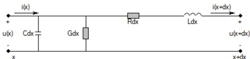
Figure 4. General transmission line model [14]
