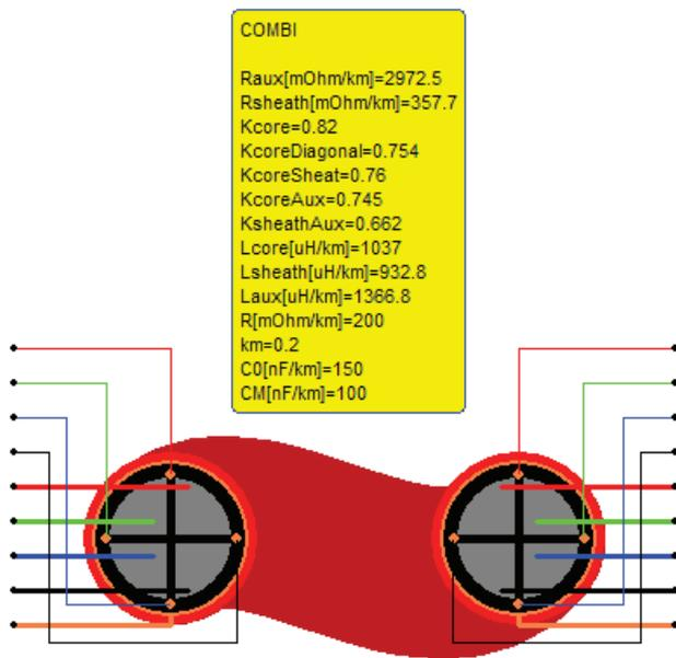
Figure 8. Final circuit model
