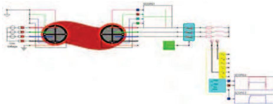
Figure 11. A load on the AC grid is connected. Scope 1 shows a voltage spike occurring in the DC grid while disconnecting the AC load on Scope 2 and 3.
