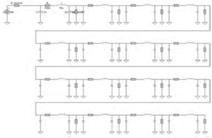
Figure 7. CombiCable model represented by 16 PI sections
