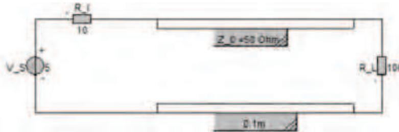
Figure 5. Simulation test circuit for reflection measurement
