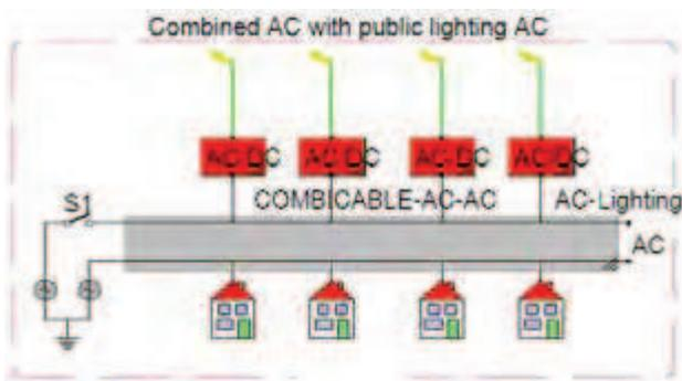
Figure 2. Distribution system using AC[13]
