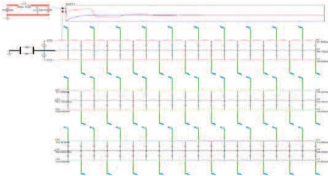
Figure 13. DC bipolar grid of 3km feeding 60 street lights at a distance of 50 meters.
