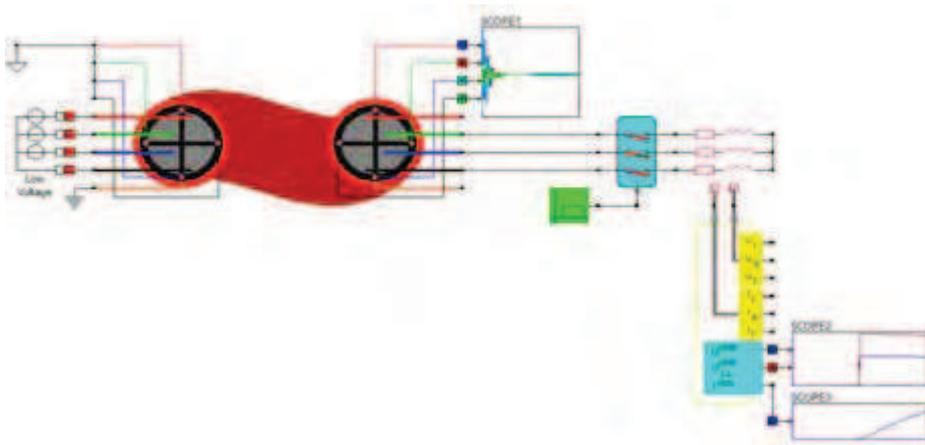
Figure 10. Simulation of disturbance in a DC grid due to switching in the AC grid.
