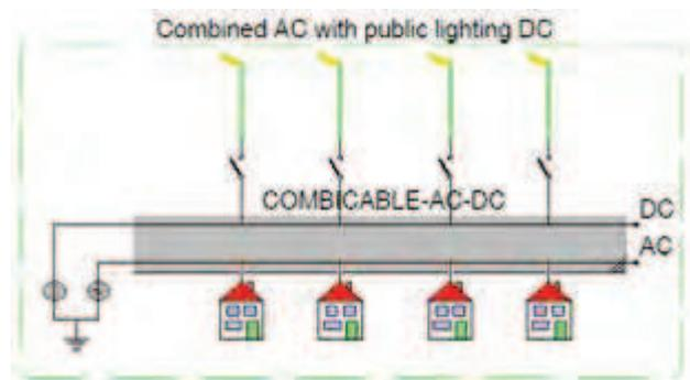
Figure 3. Distribution system using AC and DC[13]
