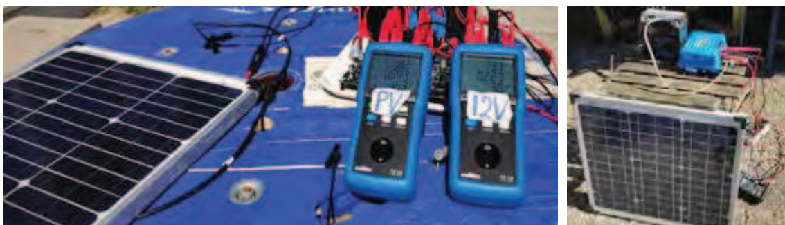
Fig. 7 The U4L tested outside compared to a test with a commercially available MPPT.
