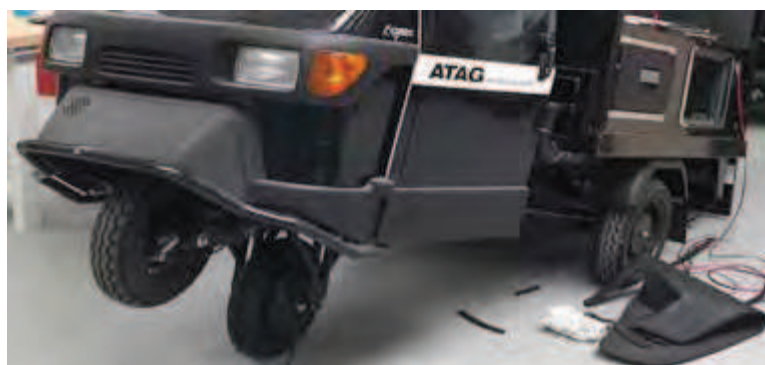
Fig. 20: The hub motor mounted for testing performance under load.
