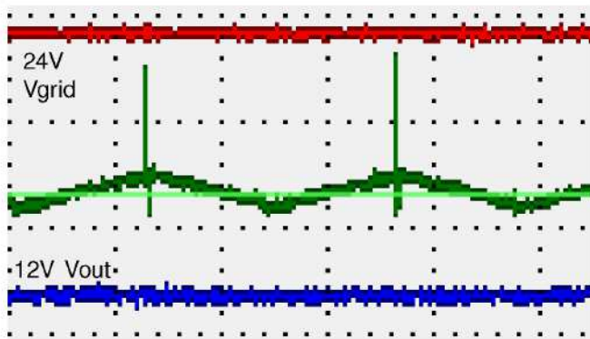
Fig. 11. Measurement showing stable voltages (Red: 24V DC, Blue: 12V DC, 5V/div) and a triangle-wave current flow (Green: 1A/div, 10 \mu s/div)
