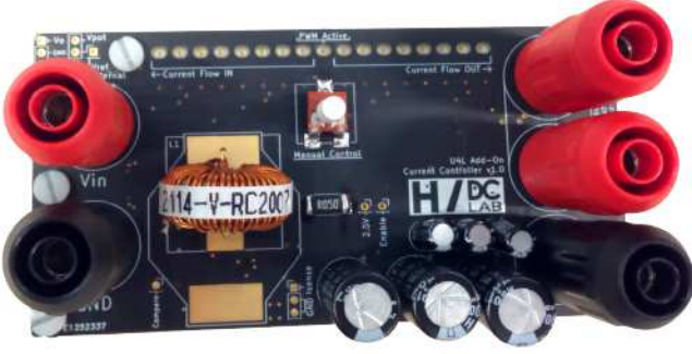
Fig. 7. Fully assembled current controller [18]. The connectors on the left side match the connectors on the U4L. The application is connected to the connectors on the right side.
