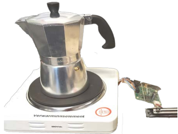
Fig. 15. DC grid (+350V) supplying a resistive heater with a current regulated circuit. The circuit is limited on a 1kW load.
