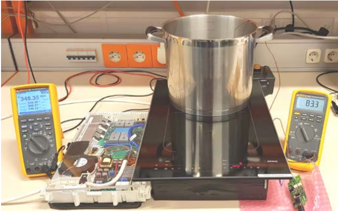
Fig. 12. DC grid (+350V) supplying an inductive cooker. The circuit is limited on a cooking level of 1kW.
