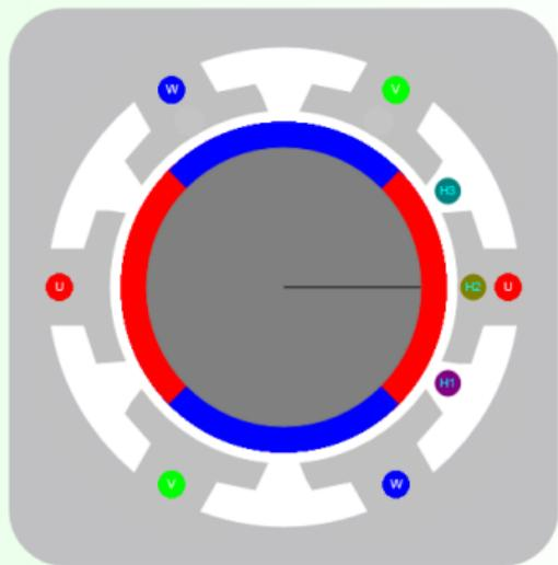
Rotor angular position  $\theta_m=0^\circ$
